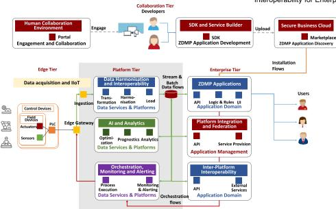
The ZDMP architecture has four tiers, each composed of several components: Collaboration Tier (design-time); Enterprise Tier (usetime); Platform Tier (run-time); and an Edge Tier (distributed runtime). All tiers except the Collaboration Tier, are based on the RAMI4.0 (Reference Architectural Model Industrie 4.0) architectural model:
